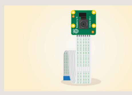
The Raspberry Pi camera module v2 replaced the original camera module in April 2016. The v2 camera has a Sony IMX219 8-megapixel sensor (compared to the 5-megapixel OmniVision OV5647 sensor of the original camera).
