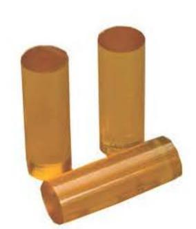
3M™ Hot Melt Adhesive 3779 Q is a 100% solids thermoplastic, high heat resistant adhesive. Good electrical properties for potting and wire tacking. UL 94 V-0 Listing.
