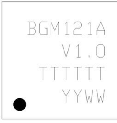
Figure 8.4. BGM121/BGM123 Package Marking
