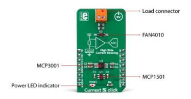
The similar schematic could be designed using only operational amplifiers, however due to a high inaccuracy of such design (as the offset voltage of a typical operational amplifier can greatly affect the output current, especially after the amplification is applied), and the low common mode voltage that typical operational amplifier can withstand, specialized current sensing amplifier ICs (CSA) such as the FAN4010, are used instead.
