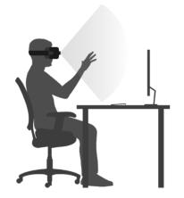
The Leap Motion Controller features a 120×150° field of view and an interactive tracking range of more than 2 feet (60cm).
