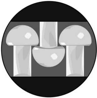
Mushroom-shaped heads slide over each other and snap together
