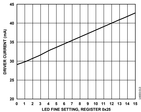
Figure 16. LED Driver Current vs. LED Fine Setting (Coarse Setting = 0x0)
