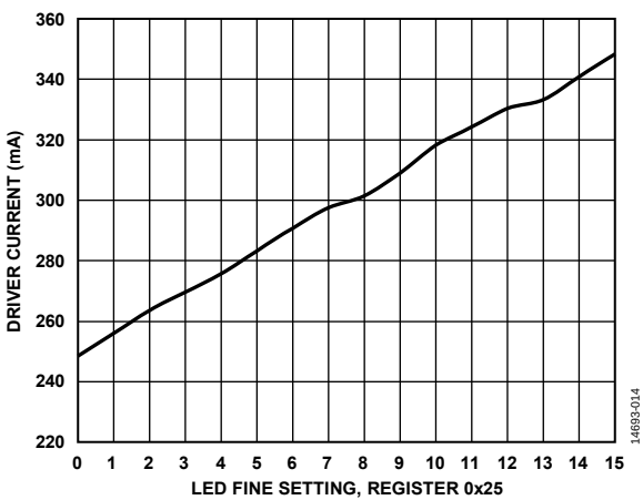
Figure 17. LED Driver Current vs. LED Fine Setting (Coarse Setting = 0xF)
